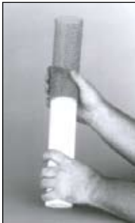
(L-r) Place plastic loading slats over filter. Then slide web over slats and pull down. Remove slats and cartridge is ready to reuse.
