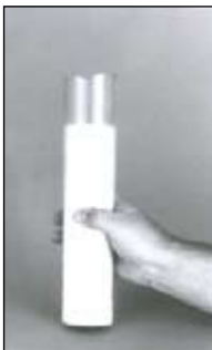
(L-r) Place plastic loading slats over filter. Then slide web over slats and pull down. Remove slats and cartridge is ready to reuse.
