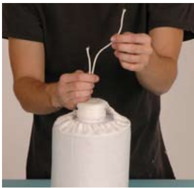
Fig. 6. Pull string on right side of bag about 3" longer than on left.
