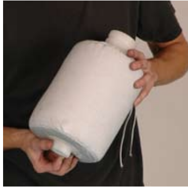
Fig. 1. Insert filter cartridge into bag and tighten nut at bottom.
