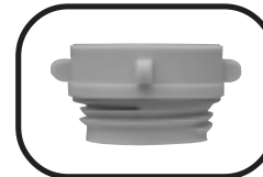
Containers with coarse (Buttress) threads require Buttress Adapter for proper seal: 2.5"-diameter (63-mm) adapter fits most U.S. drums. Use 2.25" (57-mm) adapter for most Asian and 2.75" (70-mm) for most European drums.
